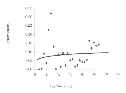
Fig 2: Semivariogram for hydraulic conductivity of soil at 15-30cm depth
