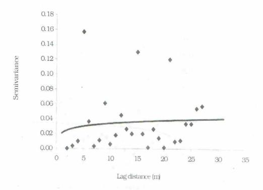
Fig 3: Semivariogram of hydraulic conductivity of soil at 30-60cm depth
