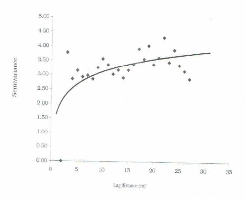
Fig 1: Semivariogram for hydraulic conductivity of soil at 0-15cm depth
